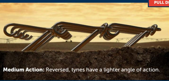
**Medium Action:** Reversed, tynes have a lighter angle of action.
